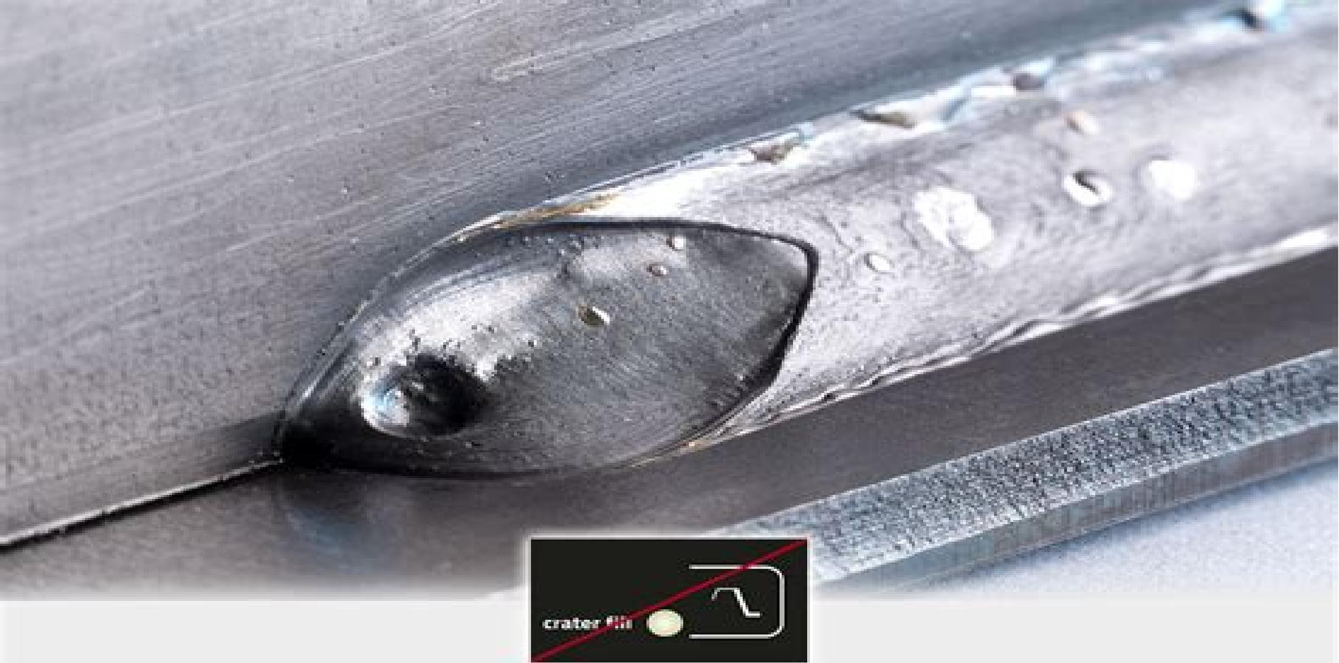
An end-crater is caused by the three-dimensional transfer of heat at the end of the weld seam, which forms an indentation. The indentation develops due to shrinkage which in turn leads to shrinkage stress. This can result in cracks in the end-crater and ultimately in the seam.
